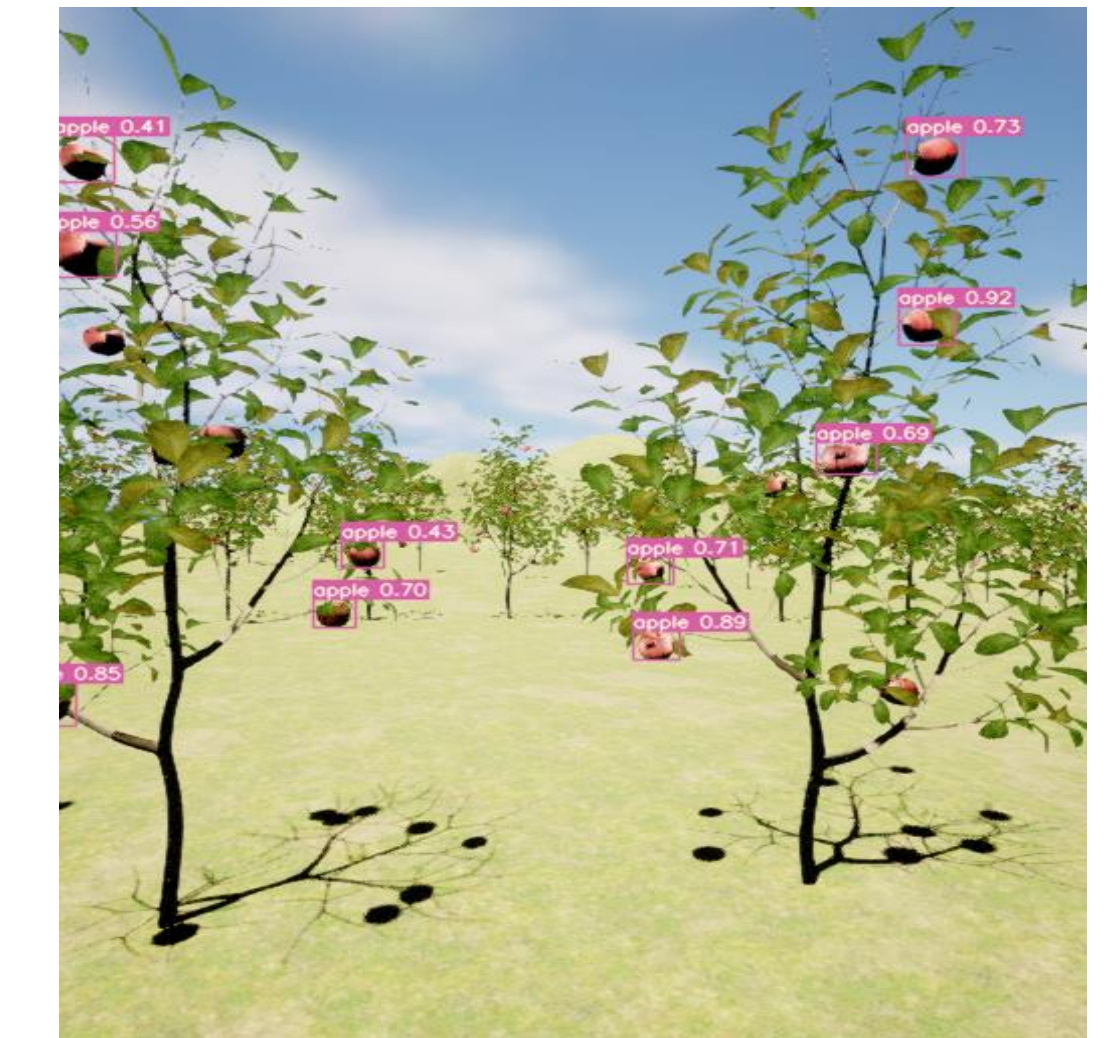
YOLOv7 apple detection on simulation
